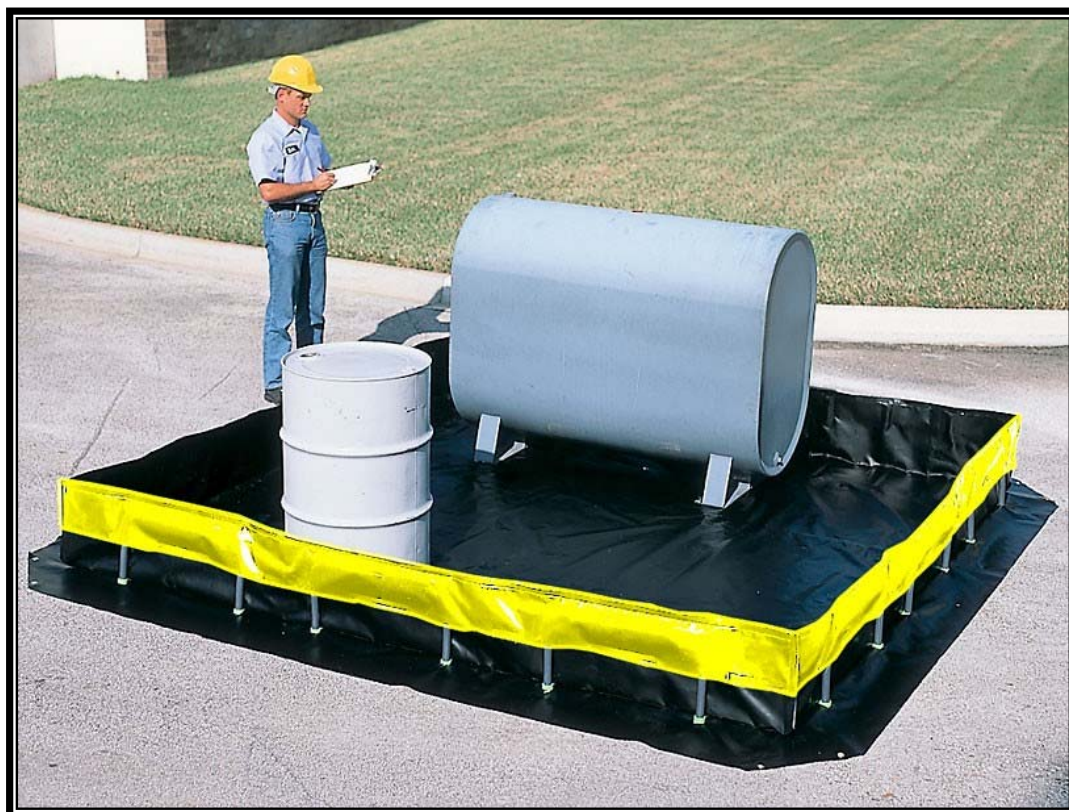
Figure 5.6. Temporary Spill Containment.
