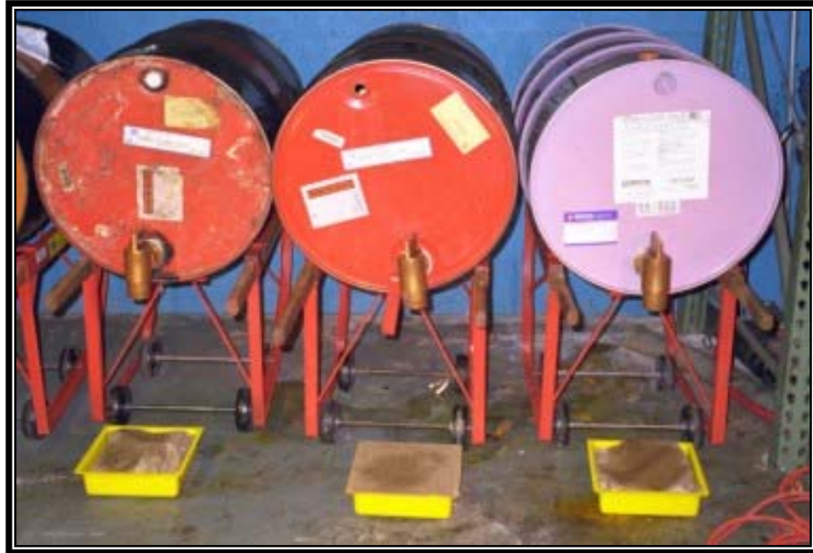
Figure 4.18. Mounted Containers with Drip Pans.
