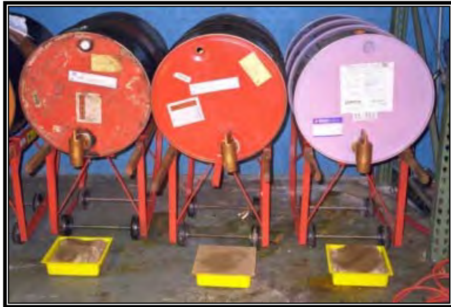
Figure 4.18. Mounted Containers with Drip Pans.
