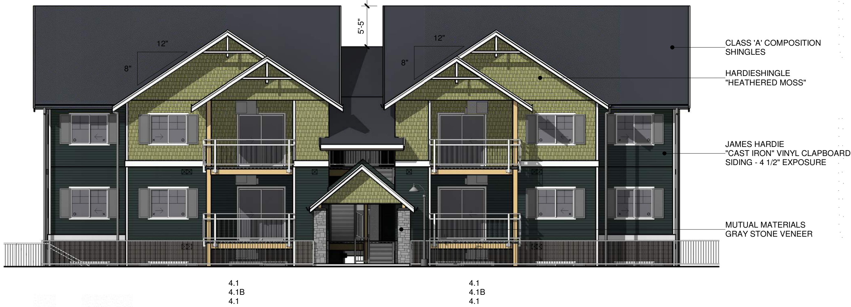
BUILDING 'C' - FRONT ELEVATION - NORTH 1/8" = 1'-0"
