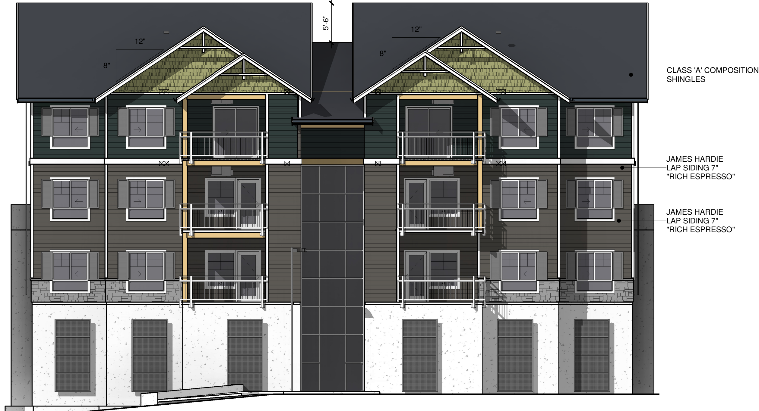
BUILDING 'E' - REAR ELEVATION - WEST
