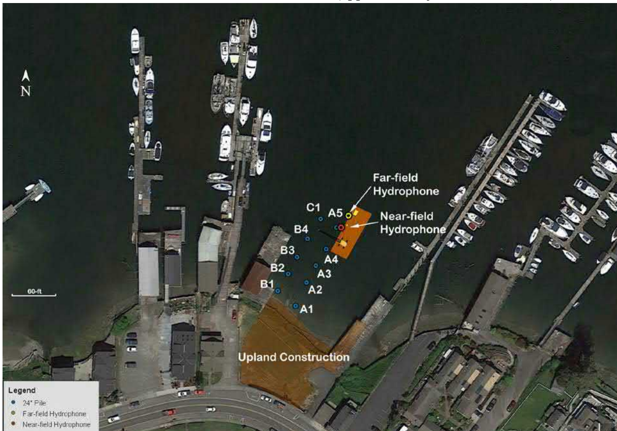
Figure 3 Ancich Pile Driving - Location of piles and hydrophones on barge.
