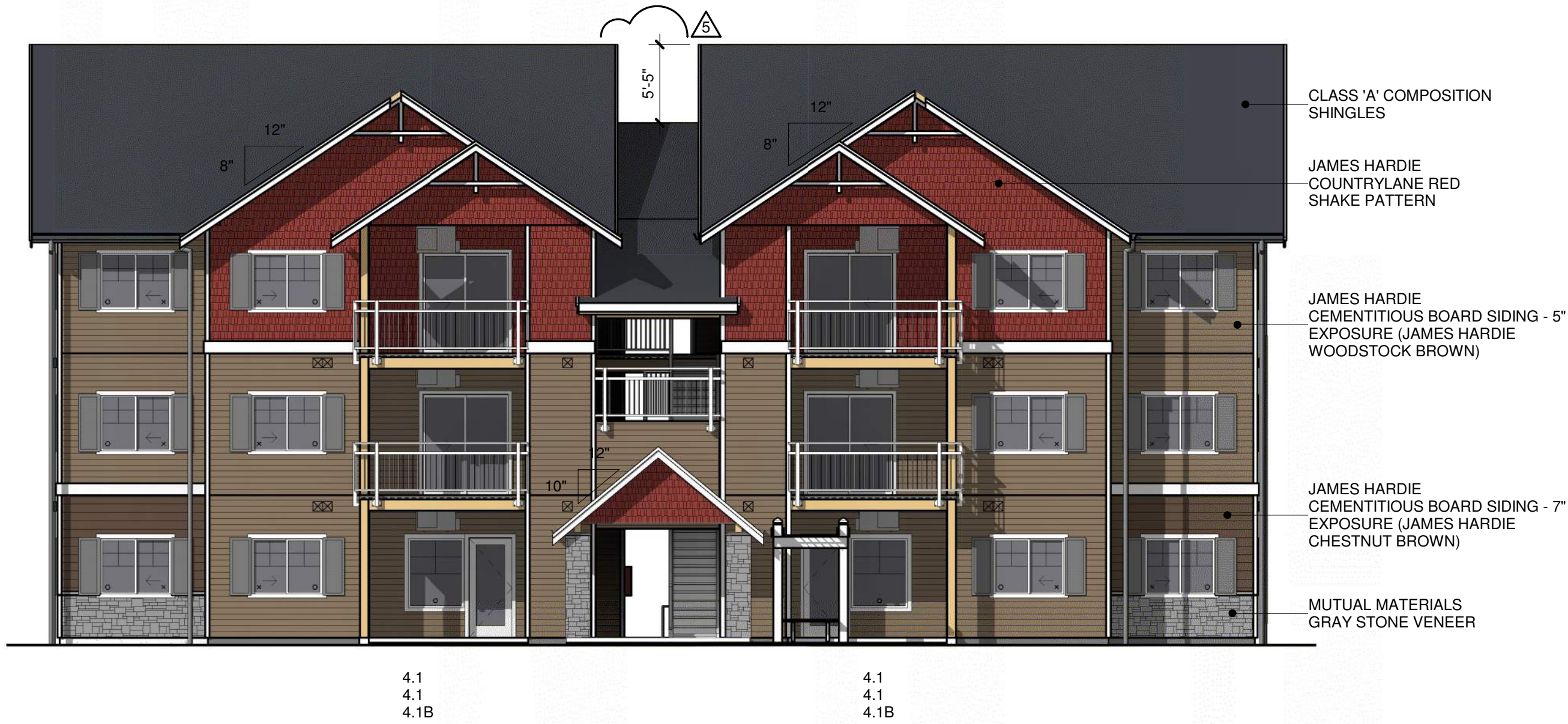
BUILDING 'D' - FRONT ELEVATION - NORTH 1/8" = 1'-0"
