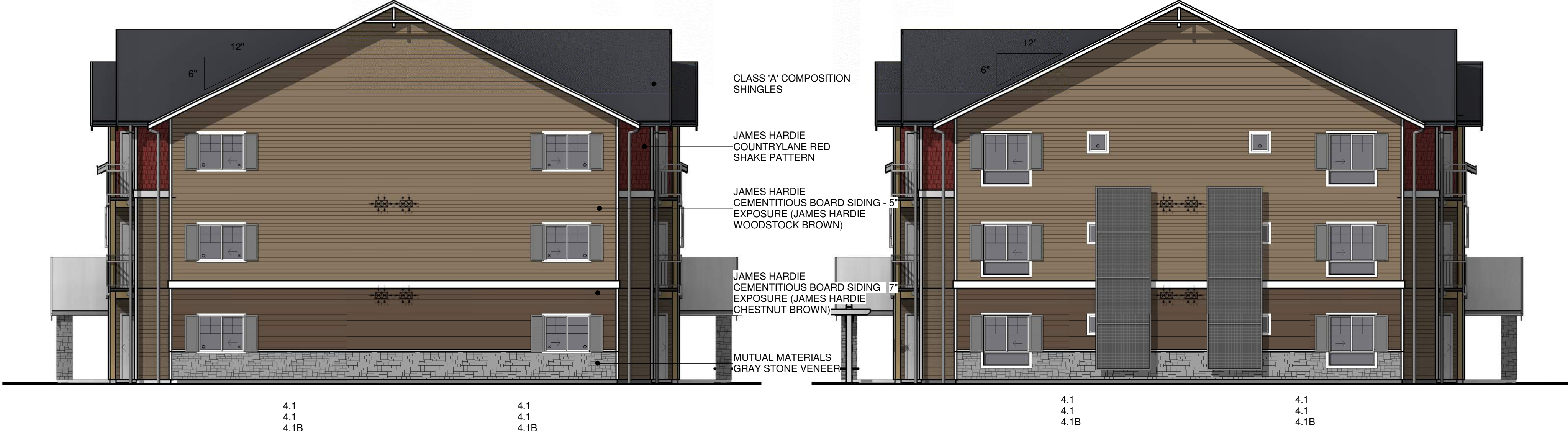
BUILDING 'D' - LEFT ELEVATION - EAST 1/8" = 1'-0"
