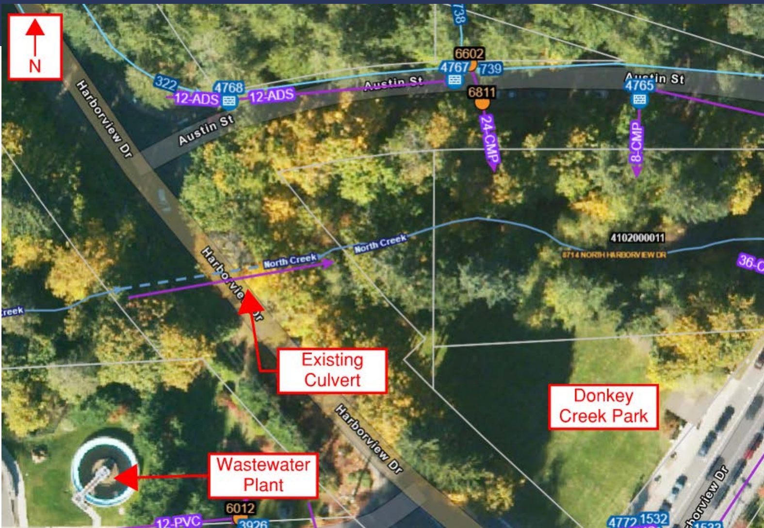
6' X 6' X 146' box culvert (constructed 1970) cataloged as 67% fish barrier by WDFW
