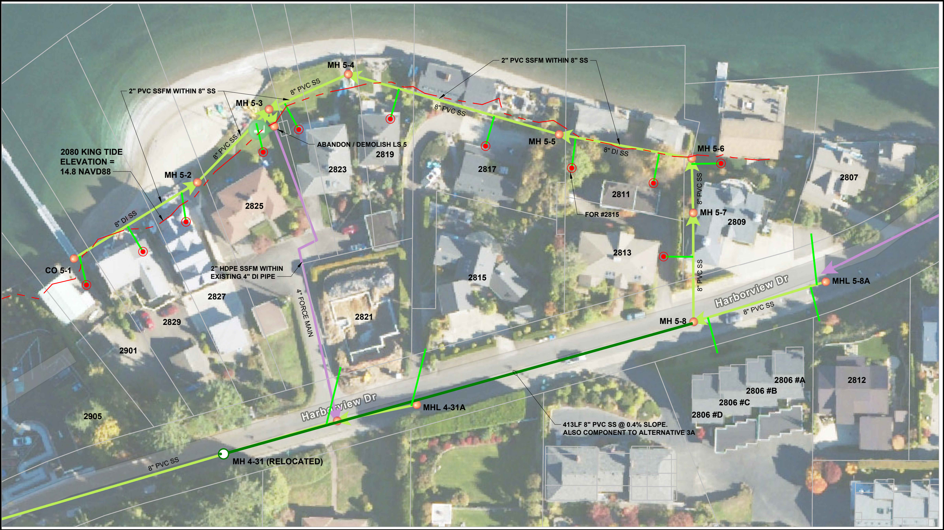
Figure 2A - Lift Station 5 Alternative 2: Grinder Pump Stations City of Gig Harbor, Washington
