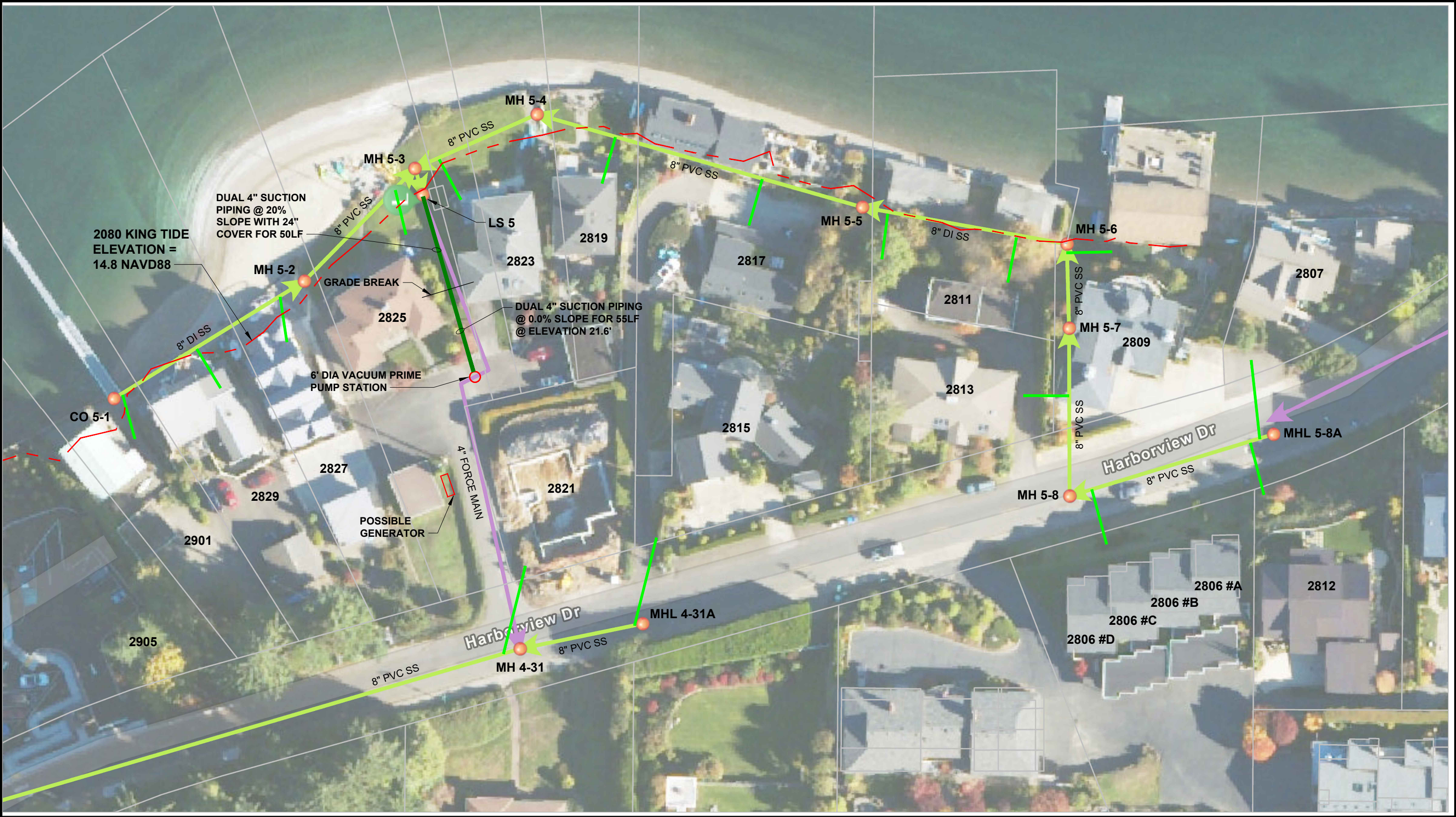
Figure 5A - Lift Station 5 Alternative 5: Relocate Duplex Vacuum Prime Pump Station City of Gig Harbor, Washington
